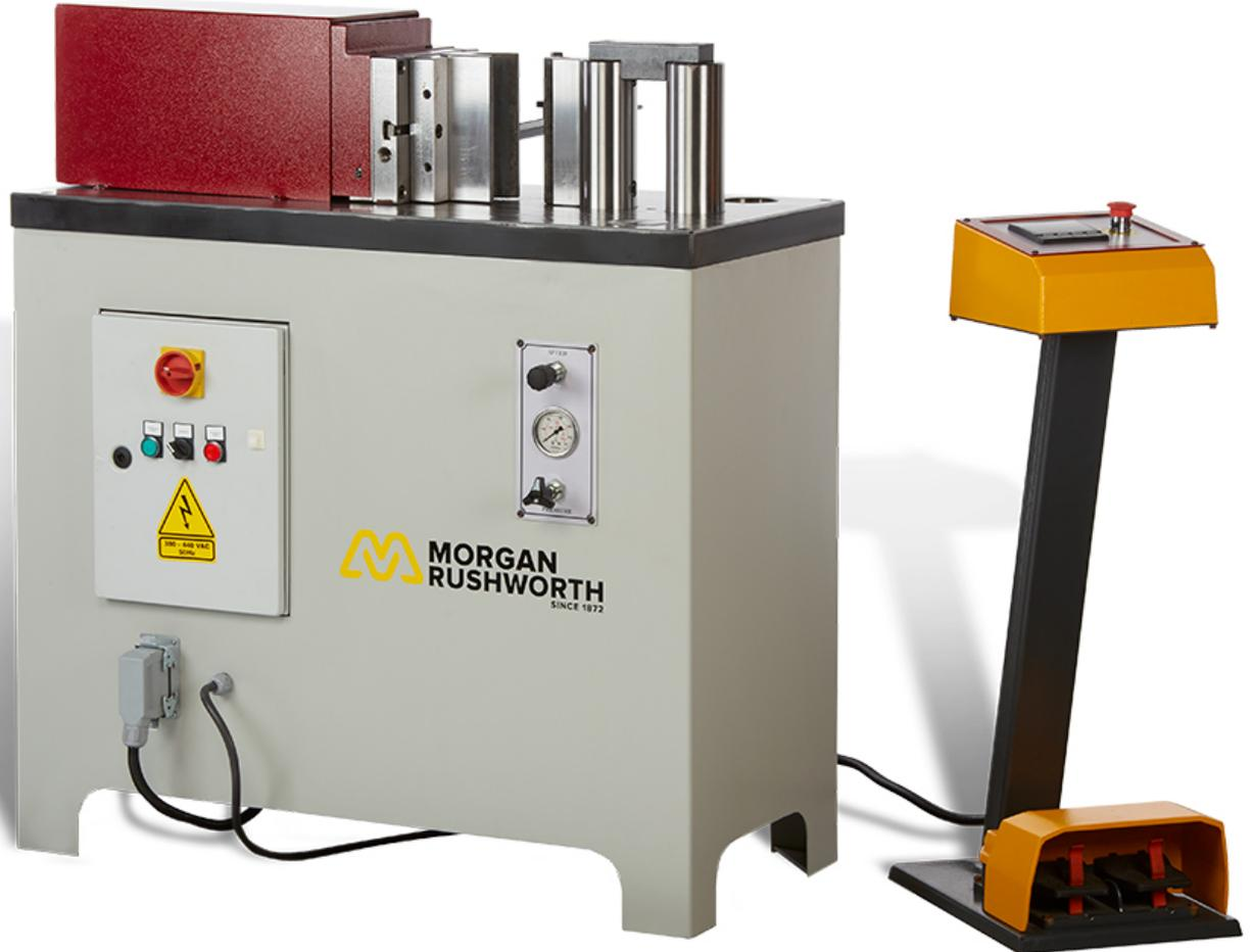
The Morgan Rushworth hydraulic horizontal bending machines are ideal for precision bending, straightening, punching and shearing. Available with capacities from 10 tonnes up to 100 tonnes and with a large range of optional tooling, these machines are capable of performing a whole variety of bending operations. The bending stroke and ram return positions are set using a simple digital programmer. Standard tools for bending flat bars are included.
